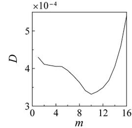
Fig. 4. Dependence  $D(m)$  for the Hutchinson system at a 5% dynamical noise.
