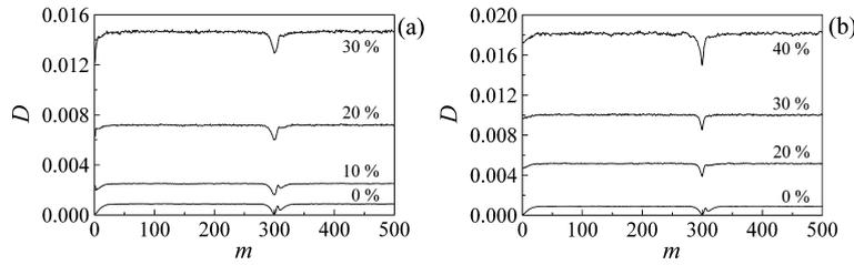
Fig. 2. Dependences  $D(m)$  for the Mackey-Glass system in the chaotic regime for different levels of additive noise (a) and dynamical noise (b). The levels of noise are indicated in % near the corresponding curves.
