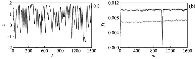
**Fig. 5.** (a) The time series of Eq. (11) with quadratic nonlinearity in the chaotic regime. (b) Dependences  $D(m)$  constructed under the assumption that the model equation is of the first order (black color) and the second order (grey color).
