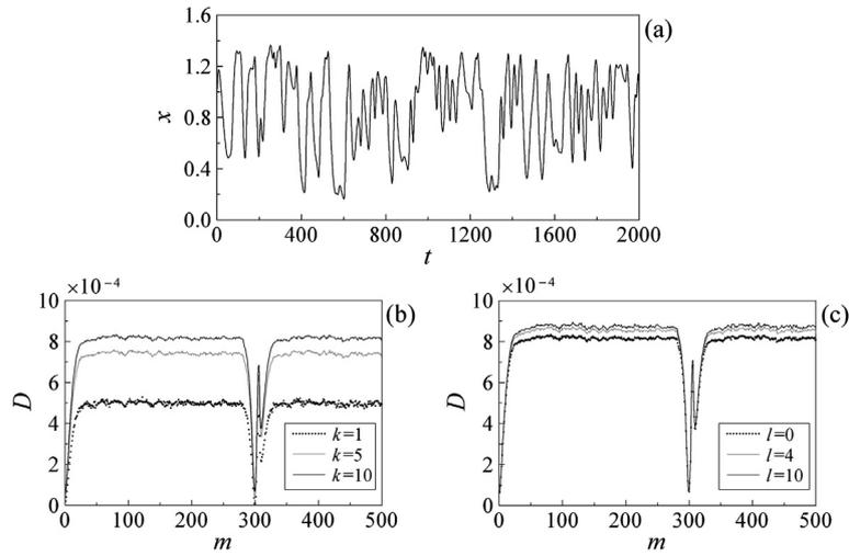
**Fig. 1.** (a) The time series of the Mackey–Glass equation in the chaotic regime. (b) Dependences of  $D$  on the trial delay time  $m$  for different numbers  $k$  of nearest neighbors. (c) Dependences  $D(m)$  for different numbers  $l$  of close in time vectors excluded from consideration.
