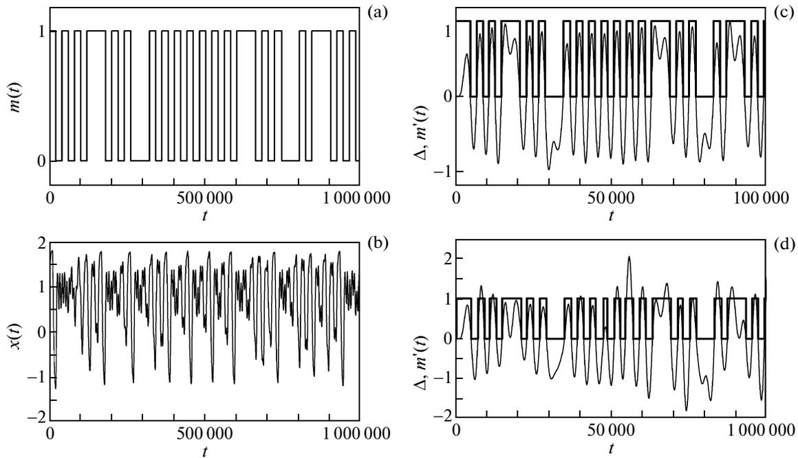
**Fig. 2.** Operation of the proposed system of hidden data transmission as illustrated by fragments of (a) time series of informative binary signal  $m(t)$ ; (b) time series of the transmitted chaotic signal  $x(t)$  in the communication channel; (c) time series of  $\Delta(t)$  signal (thin solid curve) and  $m'(t)$  signal (thick solid curve) in the absence of noise, and (d) same time series in the presence of 100% noise.
