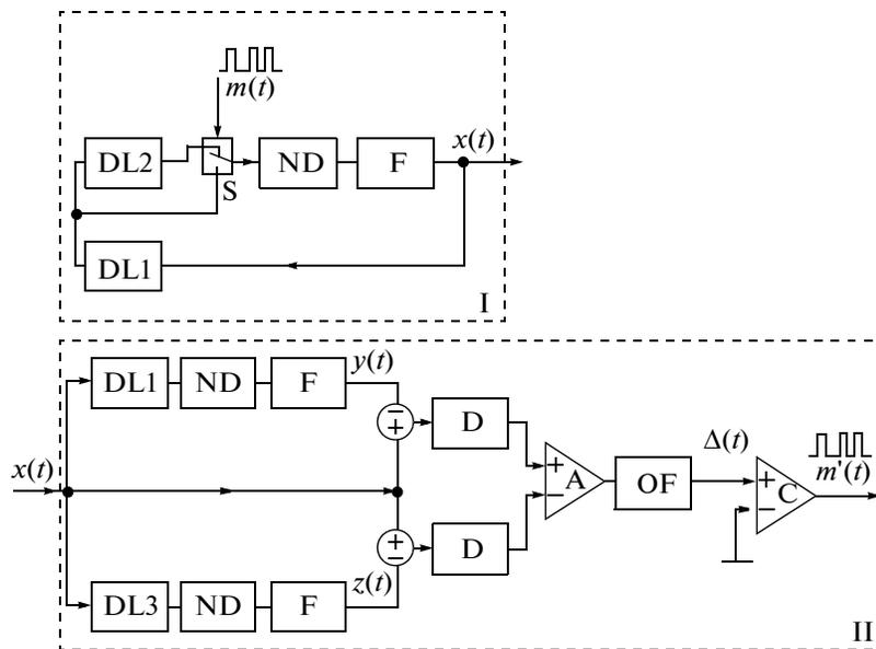
**Fig. 1.** Block diagram of the hidden data transmission system with switched delay time: (I) transmitter; (II) receiver; (DL1, DL2, DL3) delay lines; (ND) nonlinear elements; (F) filters; (S) switch (commutator); (D) detector; (A) differential amplifier; (OF) output filter; (C) comparator.
