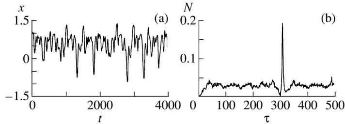
**Fig. 2.** Reconstruction of the delay time of system (2): (a) typical time series of oscillations in the system; (b) a plot of the number  $N$  of the pairs of extrema in the given time series spaced by various time intervals  $\tau$  (normalized to the total number of extrema), which shows that  $N_{\min}(\tau) = N(300)$ .
