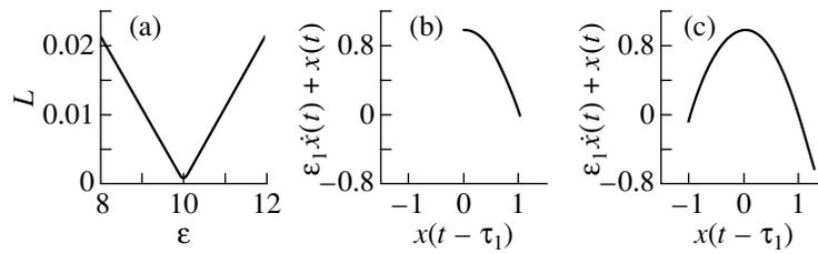
**Fig. 3.** Reconstruction of the inertial parameter  $\varepsilon$  and nonlinear function  $f$  upon the recovery of delay time  $\tau_1$ : (a) a plot of the length  $L$  of the straight segment connecting points (ordered with respect to abscissa) on the  $[x(t - \tau_1), \varepsilon \dot{x}(t) + x(t)]$  plane for  $\varepsilon$  varied at a certain step; (b, c) nonlinear functions  $f$  reconstructed from the periodic time series of systems (1) and (2), respectively.
