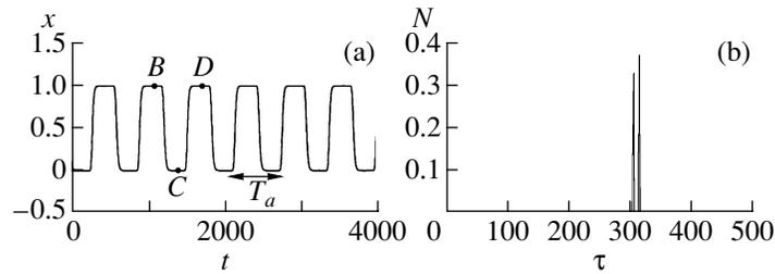
**Fig. 1.** Time-delay system (1) performing oscillations in a periodic regime: (a) a typical time series of oscillations in the system; (b) a plot of the number  $N$  of the pairs of extrema in the given time series spaced by various time intervals  $\tau$  (normalized to the total number of extrema).
