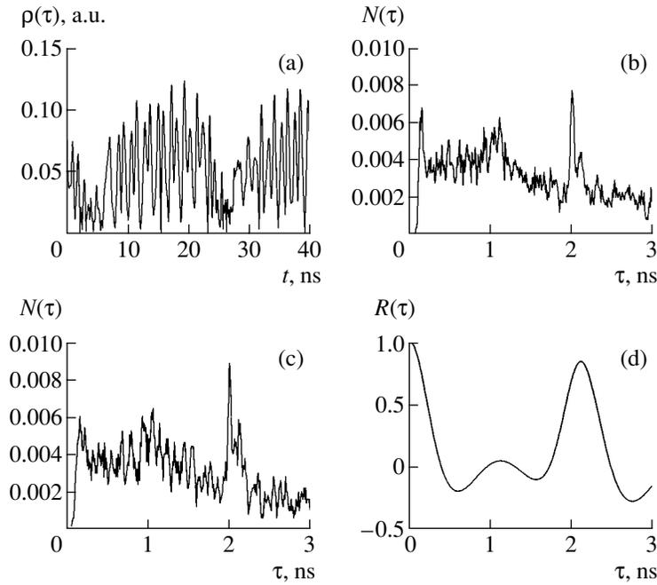
**Fig. 1.** Estimation of the parameters of a Lang–Kobayashi system (2): (a) typical experimental time series for the system with parameters  $P = 1.1 \times 10^{-3}$ ,  $\tau_0 = 2$  ns,  $\eta = 5 \times 10^{-3}$ ,  $T = 10^3$ , and  $\alpha = 5$ ; (b, c) plots of  $N(\tau)$  for the time series of variables  $\rho$  and  $I$  normalized to the total number of points simultaneously obeying conditions (4) and (6); (d) autocorrelation function  $R(\tau)$  for the laser intensity oscillations.
