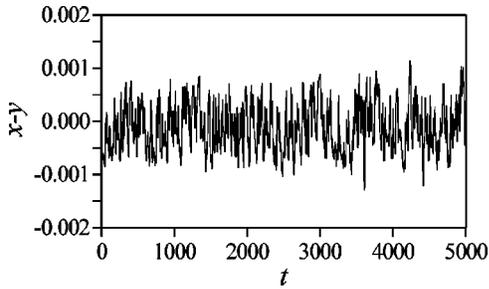
FIG. 7. The noise of desynchronization of the transmitter (2) and the recovered receiver (3) in the absence of information signal.
