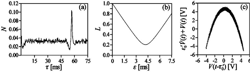
FIG. 10. Reconstruction of the electronic oscillator with delayed feedback for the case of nonlinear mixing of its chaotic signal and harmonic signal. (a) The  $N(\tau)$  plot.  $N_{min}(\tau) = N(54.75 \text{ ms})$ , (b) The  $L(\varepsilon)$  plot.  $L_{min}(\varepsilon) = L(4.2 \text{ ms})$ . (c) The recovered nonlinear function.
