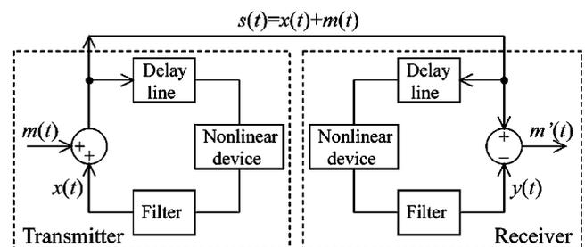
FIG. 1. Block diagram of a chaotic communication system.
