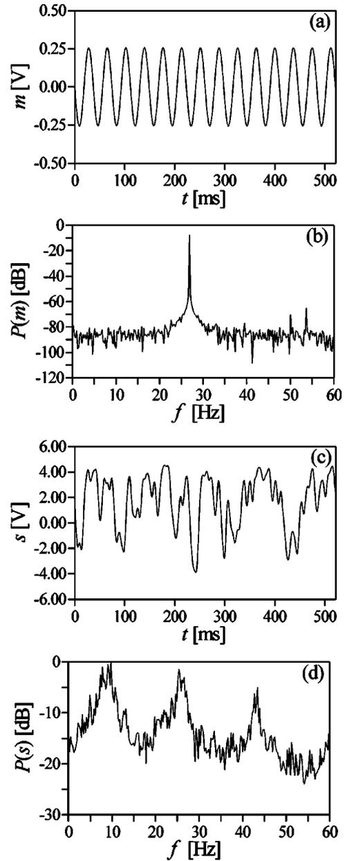
FIG. 9. (a) The original message signal with  $A = 0.25$  V and  $f_c = 27$  Hz. (b) The power spectrum of the original message. (c) The transmitted signal for  $\tau_0 = 54.7$  ms and  $RC = \varepsilon_0 = 4.215$  ms. (d) The power spectrum of the transmitted signal.
